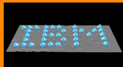
In 1989 IBM used the scanning tunneling microscope to write the letters IBM with 35 atoms of Xenon.
